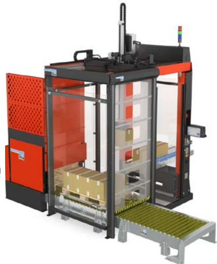
Robot palletiser with pallet magazine and automatic pallet exchange
