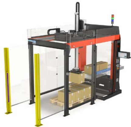
Robot palletiser, pallet on the floor, light curtain
